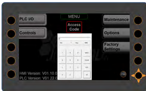
Figure 5-9 Access code keypad
