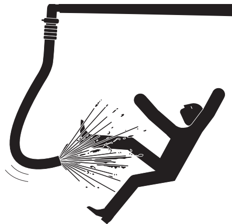
Figure 5-31 Hose whip hazard
