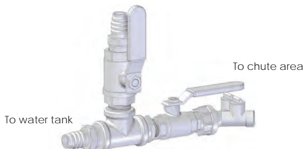
Figure 5-14 Rear water supply (Y valve)
