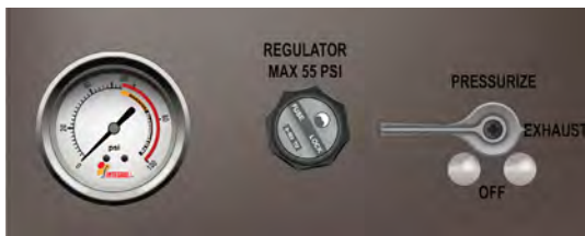
Figure 5-22 Water pressure control valve
