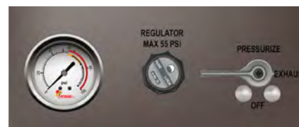
Figure 5-34 Water pressure control valve
