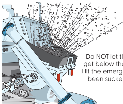
Figure 5-30 Empty Hopper Hazard
