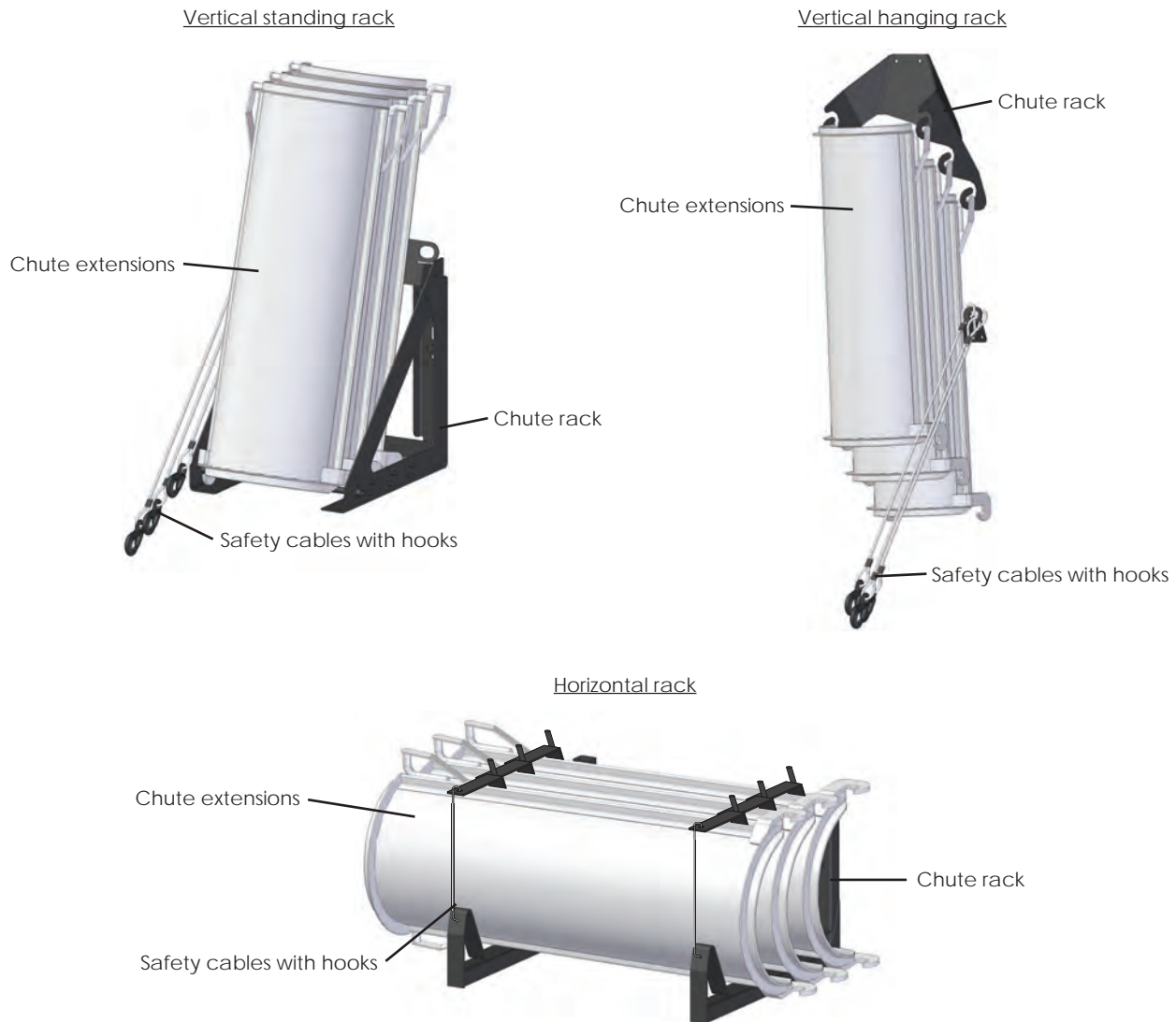
Figure 4-6 Chute rack configurations
