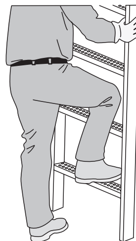
Figure 3-4 Three point rule
