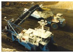
er is simple. Designed with high spiral shoulders to push the material to the drum center, and cutting teeth to properly size material, product can be loaded straight onto trucks eliminating a primary crusher, loading continuously or quickly depositing product into windrows.
