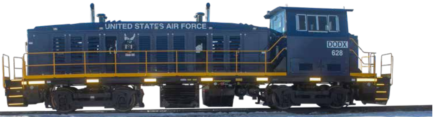
SWR18 Rear-Cab Series Switcher, Rear-mount cab 120-180 ton 1850 hp
